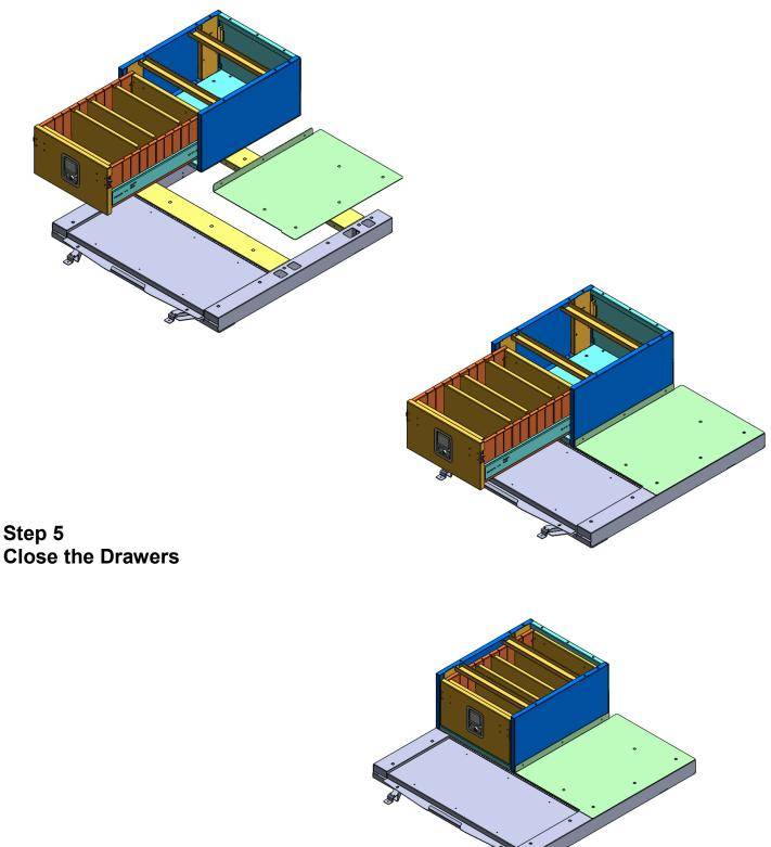
**Step 6**Replace the Cabinet Top, replace front four bolts and washers removed in Step 1.
