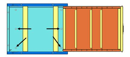
**Step 3 Place Retainer Nuts on Sub frame**
